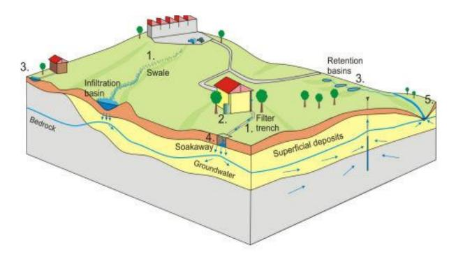
The above diagram shows the flow of water through sustainable drainage systems into the subsurface during a storm event.
